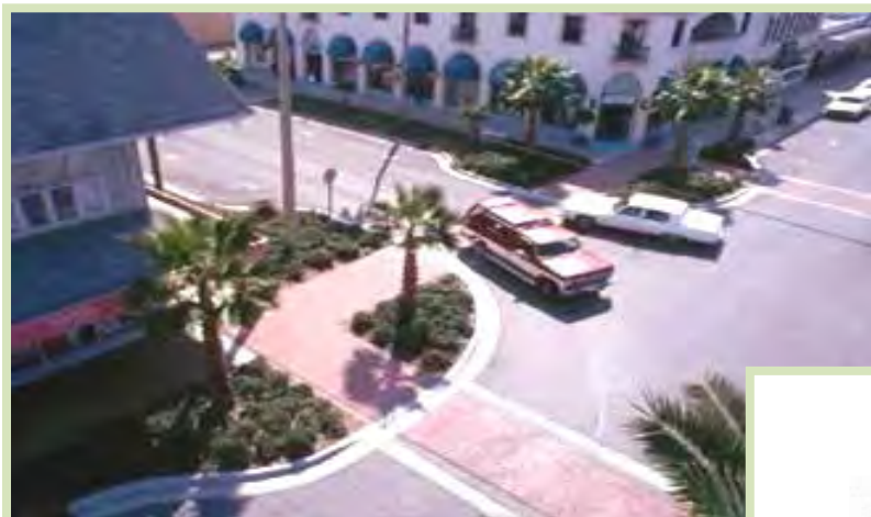
Photo and diagram illustrate features of pedestrian bulb-outs
