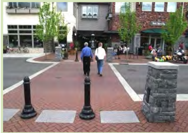
A change of materials is not always sufficient to clearly mark a crosswalk (right). The white border makes the crosswalk much more visible to drivers (left).
