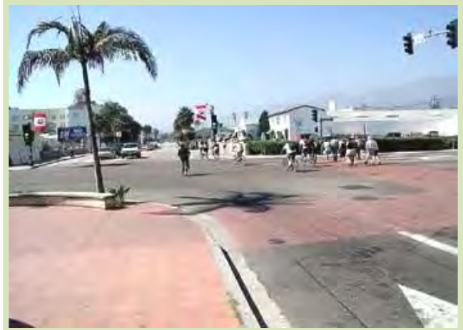
A change of materials is not always sufficient to clearly mark a crosswalk (right). The white border makes the crosswalk much more visible to drivers (left).
