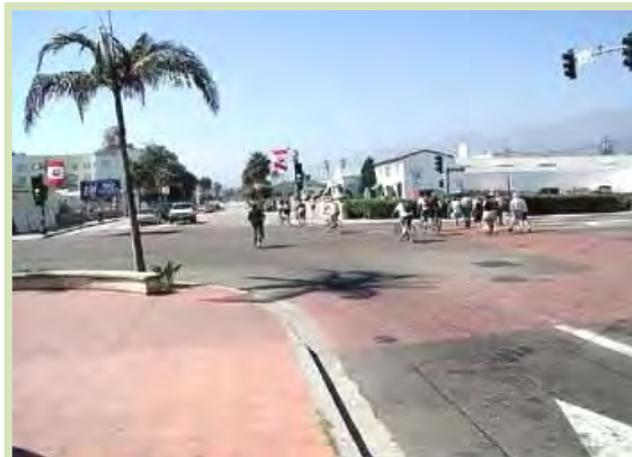
*A change of materials is not always sufficient to clearly mark a crosswalk (right).
