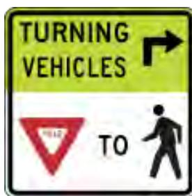
*Turning* signs are usually placed at intersections to warn motorists (that are turning right or left) to yield to pedestrians in crosswalks.
